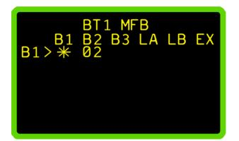
**MFB** mode is an alternative routing table being activated when the **MFB** button of a specific headset (**BT1-BT3**) is pressed. Follow the same procedure to set audio levels between sources and destinations as for the Normal mode, for each of connected headset.
